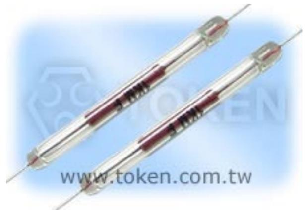
By being vacuum sealed in a glass envelope with its resistance glaze glass characteristic, these high resistance resistors are suitable for ultra-high vacuum applications, micro current circuit measurement, and pulse load equipments.
