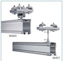
The trolleys run smoothly and quietly on plastic travel wheels mounted in anti-friction bearings that are lubricated for life. KBK trolleys feature an articulated, torque-free load connection. KBK ergo trolleys can also accommodate kick-up forces.
