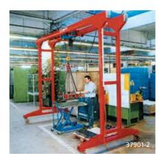
A particular advantage in many applications is that KBK portal cranes can be easily dismantled, transported and quickly re-erected elsewhere. The crane girder span can also be adjusted.
